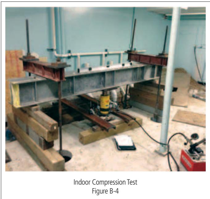
gauges (must be accurate to .001") mounted on an independent reference beam, a transit level surveying system, or other types of devices as may be specified by the engineer.
