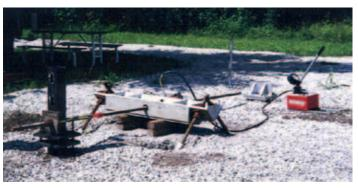
Lateral Load Test Apparatus Figure B-6
