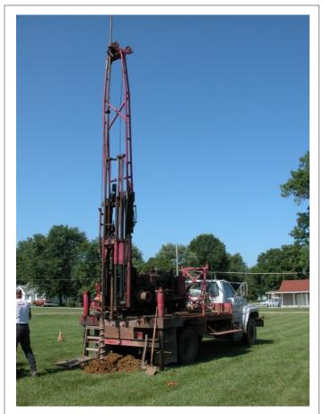
Auger Drilling Operation Figure 2-7
