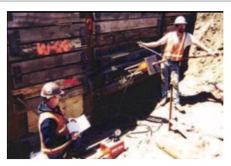
Anchor Tension Load Test in Minneapolis, MN Figure B-2
